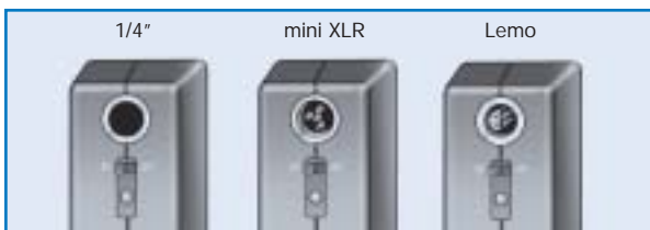
Figure 4-2: examples of input connectors
