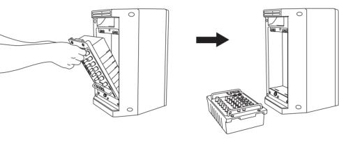
Use only the mixer's handles when removing the mixer from the speaker and when carrying the Use only the mixer's handles whe mixer separate from the speaker.
