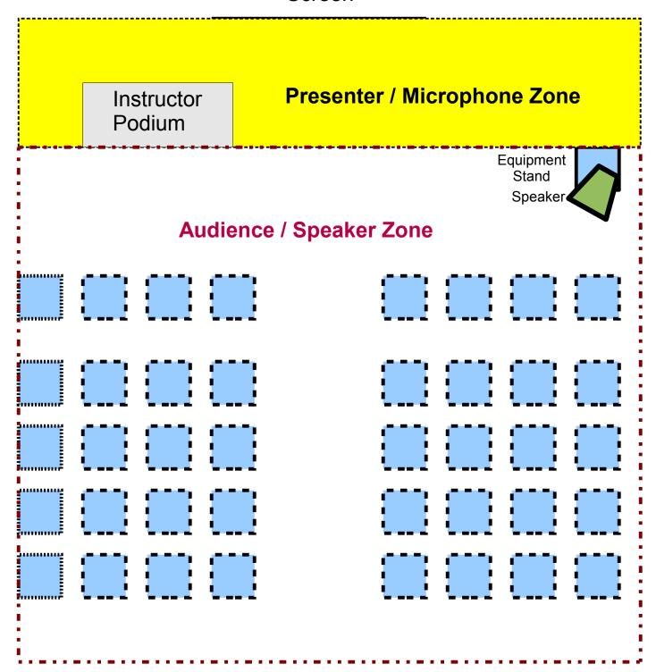
For best performance, and to avoid feedback, Presenter should stay within microphone zone. Powered speaker must be forward of Microphone Zone.
